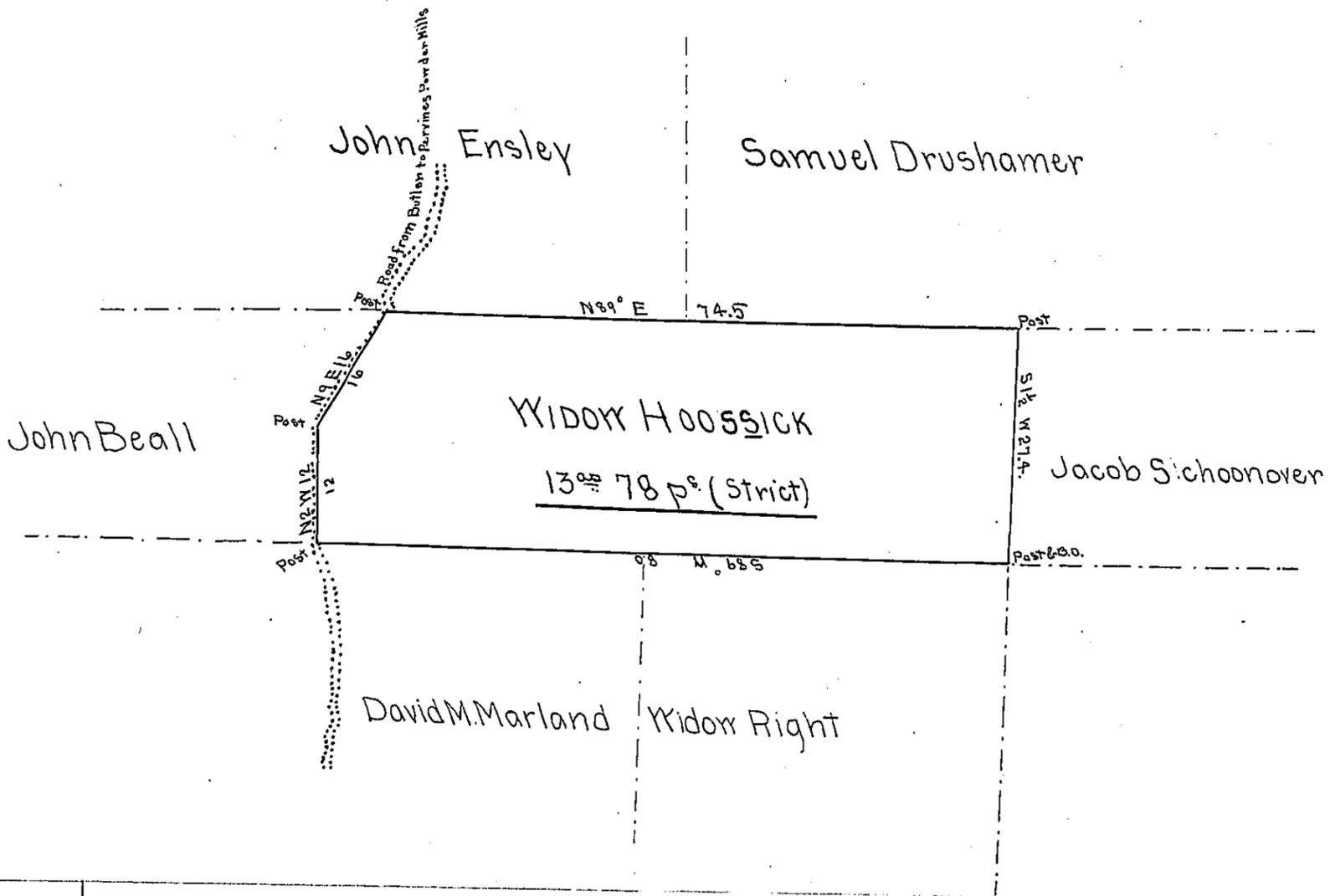
Draft of a tract of land Situated in Connoqueenessing Tp. Butler Co. Surveyed at the instance of Widow Hoosick in persuance of a Patent by Virtue of the actual Settlement and improvement. Surveyed Jan. 14<sup>th</sup> 1864. Containing 12<sup>ac</sup> 68 p<sup>s</sup> and the usual allowance of six per cent.
